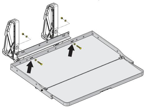
5. With the platform folded, loosely install the seat platform to the vertical support brackets using (2) M10 x 25 Hex Head Bolts, (4) Flat Washers and (2) Nylock Nuts (Bag #2).
