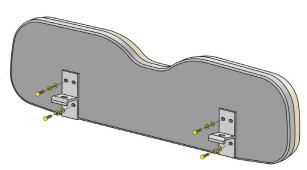
15. Install the rear seat back assembly to the rear seat back support frame using (2) M10 x 45 Hex Head Bolts, (4) Flat Washers and (2) Nylock Nuts (Bag #5).
