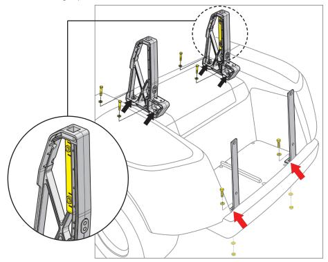
Loosely install the seat platform and seat platform support bracket to the front seat back support brackets using (2) M10 x 60 Hex Head Bolts, (4) Flat Washers and (2) Nylock Nuts (Bag #2). Install to upper hole.
