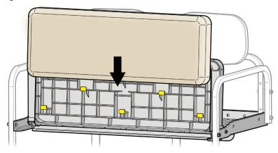
Fasten the handle to the seat platform using (2) M6 x 20 Phillips Head Countersunk Screws (Bag #5). Hand tighten to lock the seat bottom into place.
