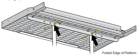
Loosely fasten the footplate to the vertical support bracket using (2)
